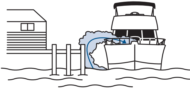
Figure 1. Blocked hull exhaust outlets near a pier, dock, seawall, bulkhead or any other structure can cause excessive accumulation of Carbon Monoxide gas with the cabin areas of your yacht. Be certain hull exhaust outlets are not blocked in any way.
