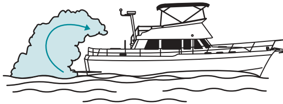
Figure 5. Engine or generator exhaust from your yacht while underway at a slow speed can cause excessive accumulation of Carbon Monoxide gas within the cabin and cockpit areas of your yacht. A tail wind can increase the accumulation. This is often referred to as the “station wagon effect”. Always provide adequate ventilation or increase your speed if possible.
